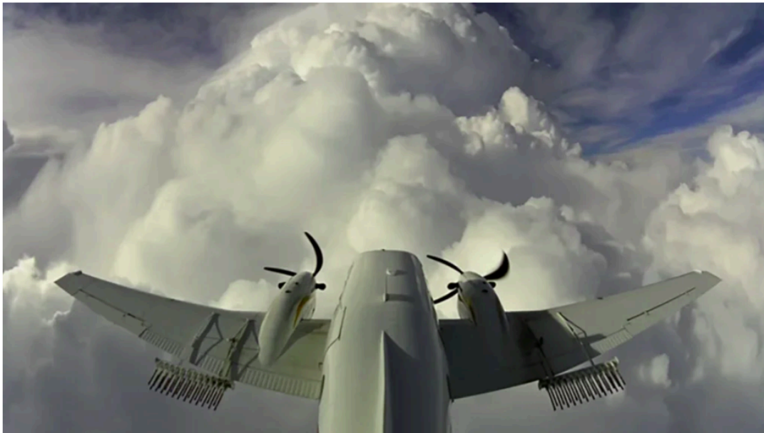
"An aircraft flies into the clouds carrying flares filled with silver iodide being released to help make more snow." -Weather Modification International 2022
